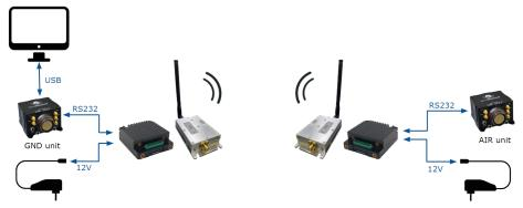
**DTC** + amplifier radios and 1x operation
