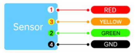
WitMotion HWT905-232 connector pinout
