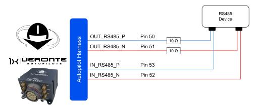
**Resistors connection between 1x and servo**
