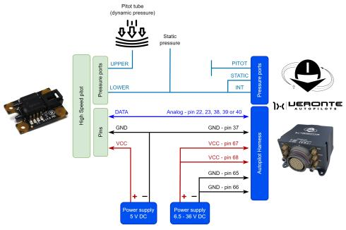
High Speed Pitot Sensor - Autopilot 1x connections diagram
