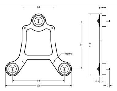
**Damping system dimensions (mm)**
