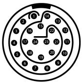
MC24 connector pinout
