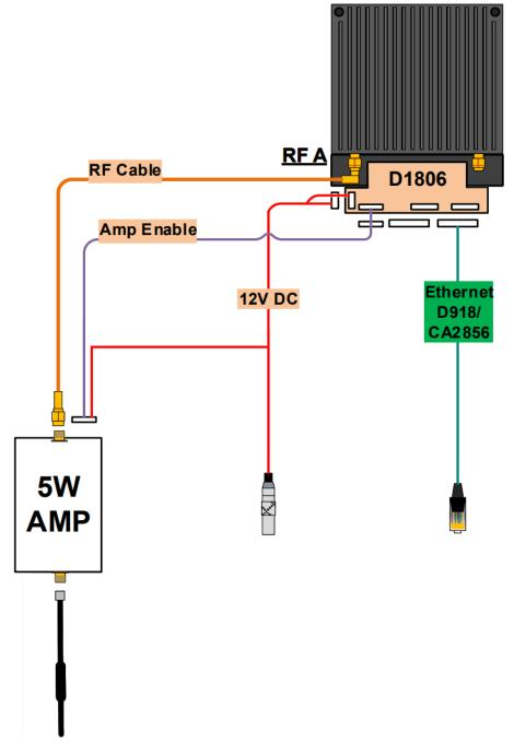
**DTC** + amplifier connection - Configuration
