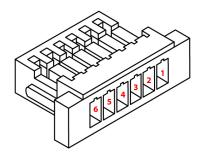
J3 (RS232) pinout of female connector
