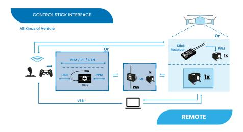
Although the most common way of control is to directly connect a **stick** via **PPM**, **RS** or **CAN** to a control station (**PCS/1x**) which then communicates with the onboard autopilot,
