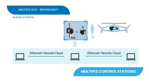
For remote solutions with LOS backup operator, **Veronte Cloud** allows the connection between PCs.
