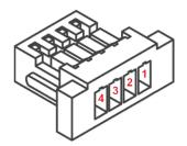
J3 (RS232) pinout of female connector
