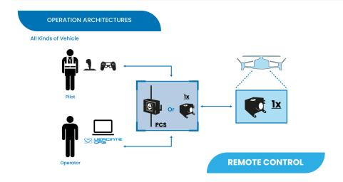
In the standard remote layout, an Operator (Internal Pilot) controls the UAV from the Ground Station using **Veronte Ops**.
