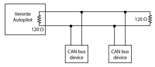
**CAN** assembly example diagram
