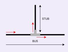
The CAN protocol specifications limit the distance a device can be placed from the BUS. The following table shows the distance limitations to be considered when setting up the system.
