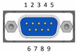
Magnetometer Honeywell HMR2300 connector pinout
