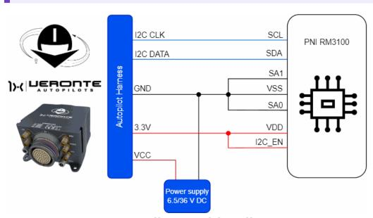
PNI RM3100-CB - Autopilot 1x wiring diagram
